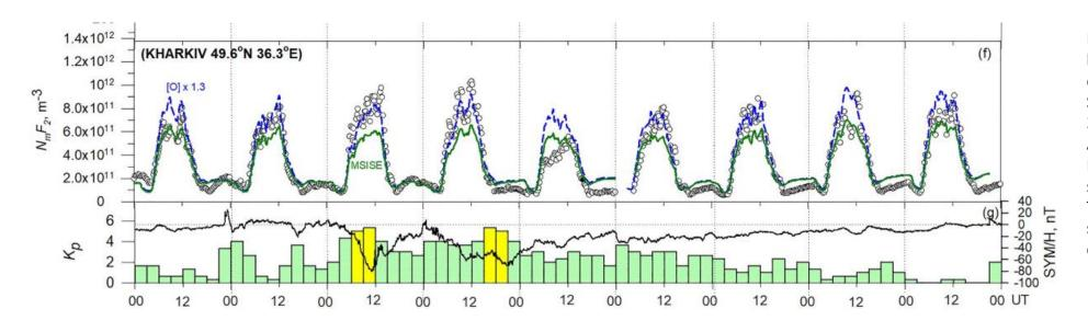
Diurnal variations of the ionosphere F2-layer peak height hmF2 and density NmF2 at Kharkiv, 3-hr Kp and SYM/H indices during 1–9 February 2022. The circles show observations. All the colored lines are from the Field Line Interhemispheric Plasma model simulations with the hmF2 constraint. The solid green line is with the standard NRLMSISE-00 densities, the dashed blue line is with a multiplier of 1.3 for the O density
